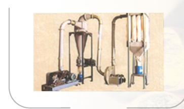
These pin mills have both discs rotating either in one direction or opposite direction. The relative speed is very critical and is maintained within design limits. The discs are rotated by two independent motors. by two independent motors. These pin mills are without These pin mills are without screen and produce fine particle size
